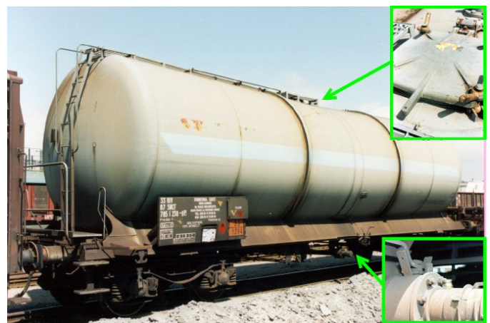
Zas tank wagon: Sealing of the roof cover and the drain valve.
